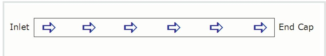
Fig. 8: Systems without AFD's offer little resistance to inflation airflow.
